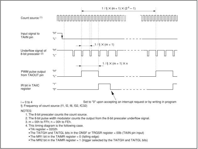
Figure 12.14 Example of 8-bit Pulse Width Modulator Operation
